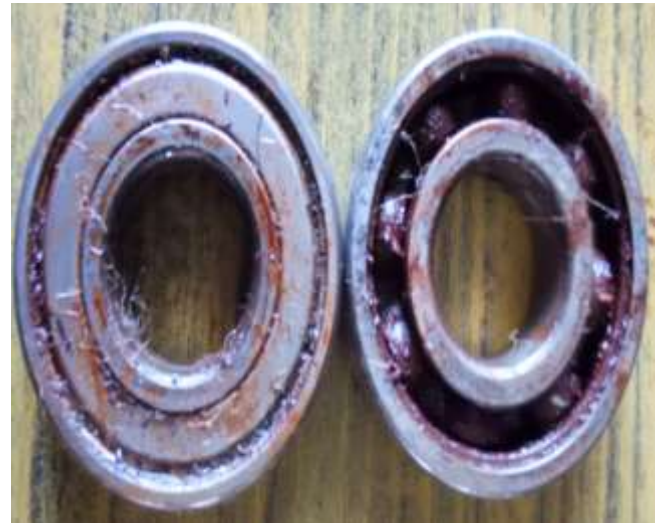
Fig 5.1 Healthy and faulty bearing
